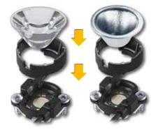
The connectors (version depends on the planned LED) and the STARboard are both fixed with two screws. Electrical contact is by means of two pushwire terminals. The optic holder is clipped onto the connector, and the optical system itself clips into this. The complete assembly process takes place without any soldering or gluing.
