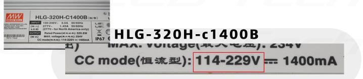
Step 1: Locate your constant current 'c' series driver's DC output voltage. this meanwell hlg-320h-c1400b has a constant current region of 114-229V DC. this means that your LED voltage must add up to at least 114V but not exceed 229V E.g. Three LOGIC boards at 45V each: 45V + 45V +45V = 135V DC. Since 135v is within the range (114-229V) this driver will power the three LOGIC pucks at a constant 1400ma.
