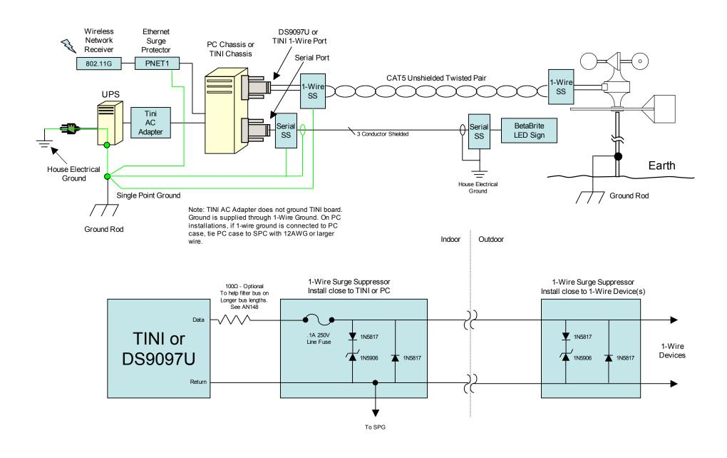
1-Wire Weather Station Grounding Technique
